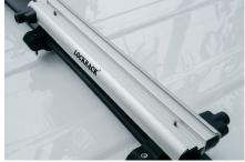
SLIDE THE T BOLT TO ALIGN WITH THE SCREW HOLES IN THE BASE.
