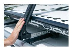
PROPERLY POSITION THE WATER CRAFT (E.G. PADDLE BOARD, KAYAK, ETC.) ON TOP OF THE BASE. IN MOST CASES, THE WATER CRAFT WILL BE UPSIDE DOWN (SUP FINS UP AND FORWARD, SURFSKI WITH HULL UP). SLIDE THE ARMS INTO THE BASE UNTIL THEY CONTACT THE WATER CRAFT ON BOTH SIDES.
