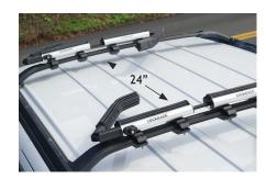
LOAD BARS MUST BE POSITIONED AT LEAST 24" OR MORE APART TO ENSURE STABILITY.
