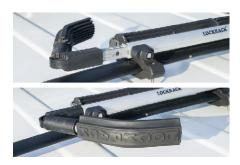
WHEN NOT IN USE THE ARMS CAN BE PLACED DOWN FOR MORE STREAMLINE AESTHETIC. DOWN TO THE LEFT IS LOCKED AND WILL NOT BE ABLE TO COME OUT, DOWN TO THE RIGHT THE ARM IS NOT IN A LOCKED POSITION AND CAN EASILY COME OUT OF ITS GROOVE. HOLE FACING LOCK SIDE, LOCKS ARM INTO PLACE (SEE TOP IMAGE).
