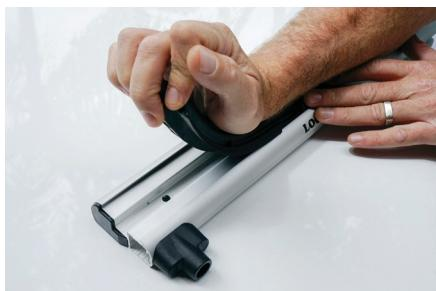
AVANT DE MONTER LA BASE SUR LES BARRES DE TOIT, ENLEVER LA PROTECTION CAOUTCHOUC DE LA RAINURE.
