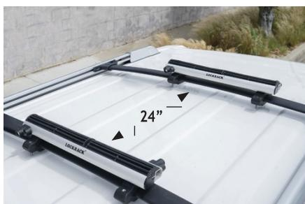
LES BARRES DE TOIT DOIVENT ÊTRE ESPACÉES D'AU MOINS 24 CM OU PLUS AFIN D'ASSURER LA STABILITÉ DU DISPOSITIF.
