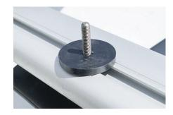
IF THE LOAD BARS ARE **EQUIPPED WITH ACCESSORY GROOVES SLIDE THE** T BOLT HARDWARE WITH THE **BLACK RING INTO THE LOAD** BAR GROOVE. IF THE LOAD BARS DO NOT HAVE GROOVES, THEN USE THE ADAPTER INSTRUCTIONS BELOW.
