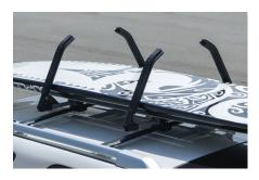
AFTER ALL 4 ARMS ARE IN LOCKED POSITION AND TIGHT GIVE THE BOARD A WIGGLE TO MAKE SURE IT IS SECURE. IF THERE IS ANY MOVEMENT, YOU MUST ADJUST THE WATER CRAFT TO PROPERLY ALIGN THE ARMS WITH THE GROOVES ON THE BASE.
