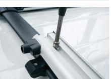
ONCE THE BASE IS PROPERLY POSITIONED ON LOAD BAR, TIGHTEN THE BOLTS WITH A 10MM WRENCH.
